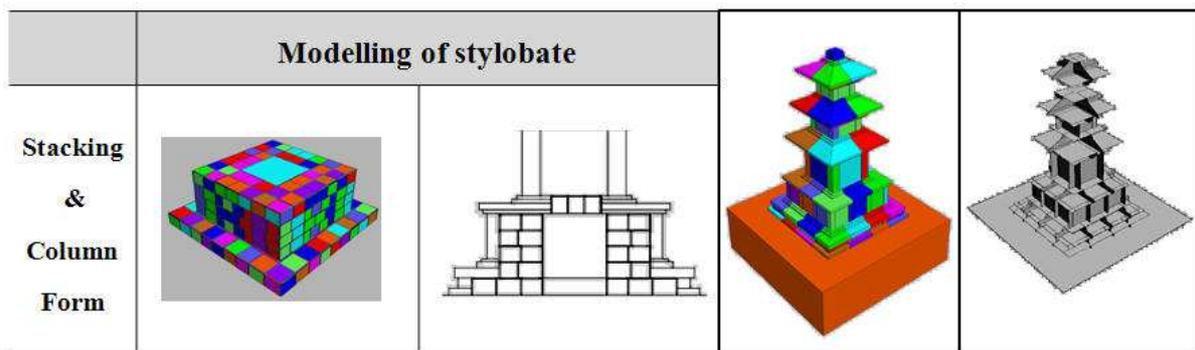
Figure 2: Structural modeling of stone pagoda
