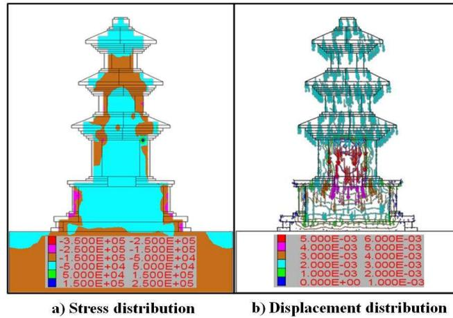
Figure 3: Stress and displacement distribution of stylobate model filled with soil
