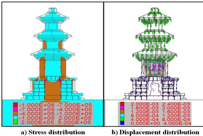
Figure 4: Stress and displacement distribution of stylobate model with column & stacking form
