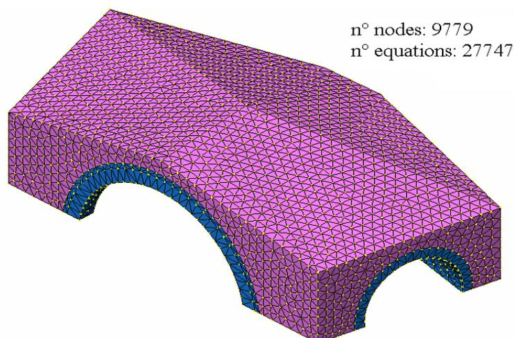
Figure 7: Finite element model of the masonry structure and of the vault-fill
