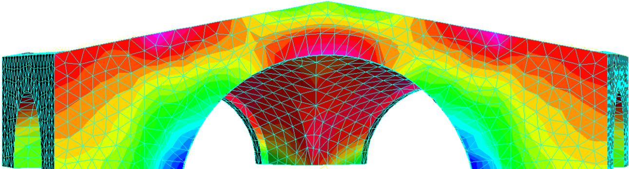
Figure 8: Colour map of normal stresses of the arch on Pallotta Canal
