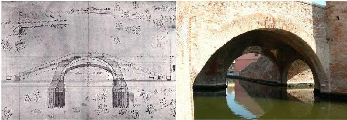
Figure 5: Longitudinal section of Pio V's bridge      Figure 6: View of the vault from Pallotta Canal
