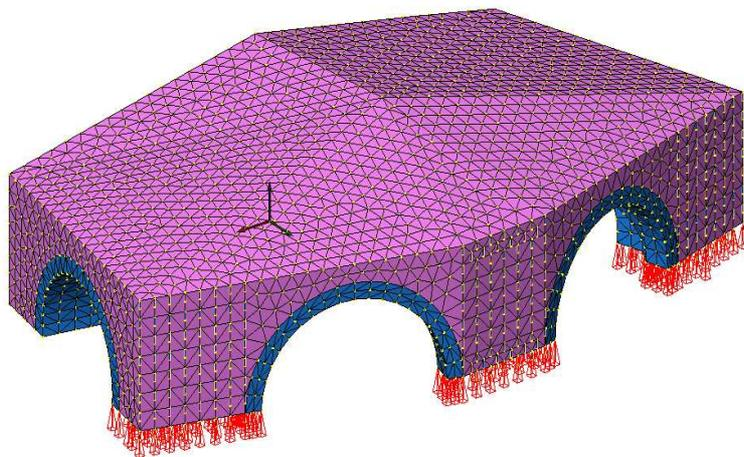
Figure 12: Finite element model employed for non linear analysis in presence of the foundation
