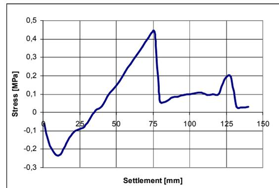
Figure 15: Stress evolution caused by the settlement
