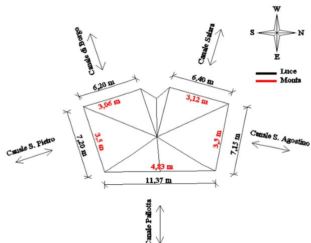
Figure 2: Geometry of the bridge's vault
