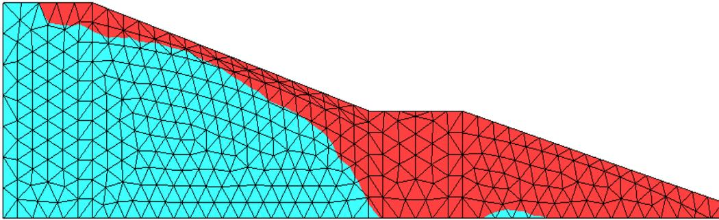
Figure 16: Colour map of normal stresses  $i \sigma_{zz}$  on North side of the central staircase
