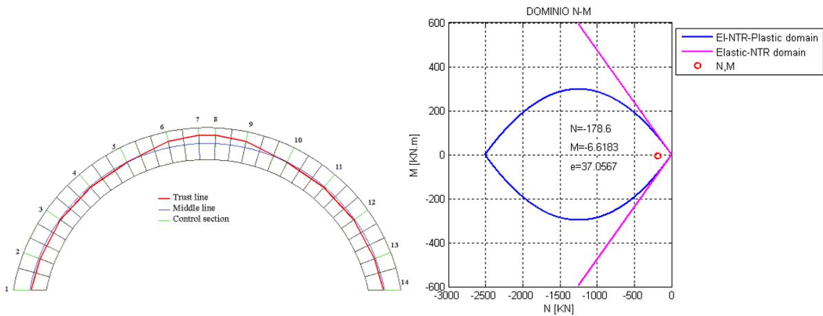
Figure 9: Thrust line of the arch on Pallotta Canal Figure 10: Domain at a section of the arch
