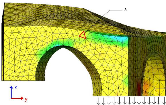
Figure 14: Colour map of the tension on the North side of the bridge FEM
