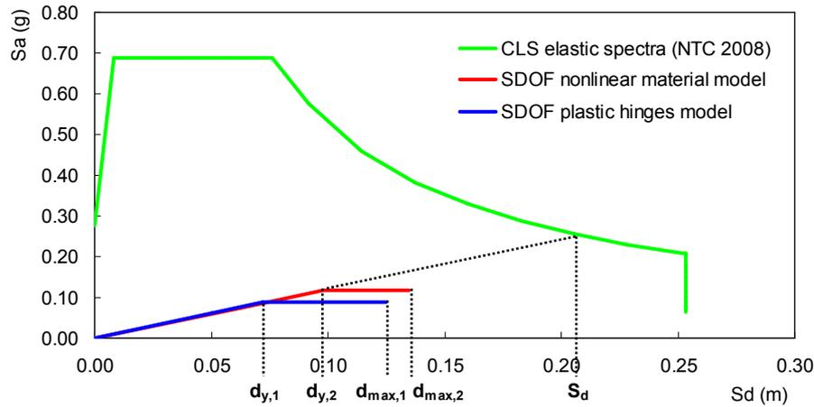
Figure 7: Capacity curves of the two considered models and seismic demand spectrum
