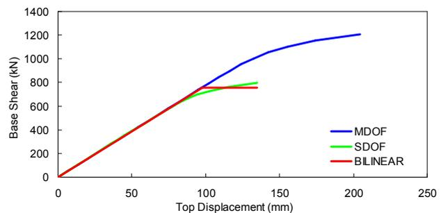
Figure 6: Pushover curve of the MDOF model, capacity curve of the equivalent SDOF system and bilinear curve
