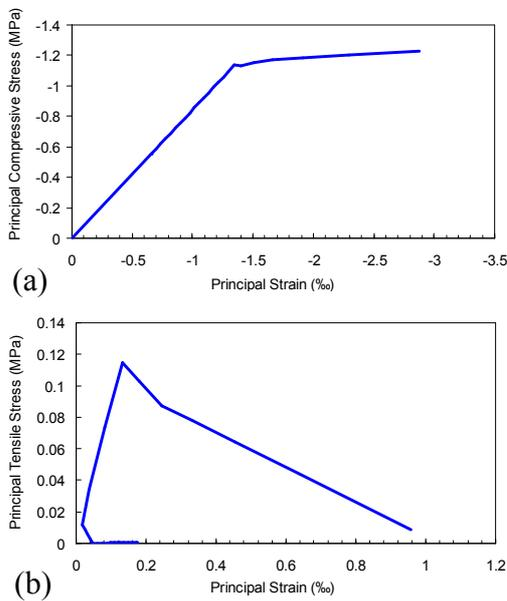
Figure 3: Principal stress-strain relation at the (a) compression and (b) tension side of the horizontal section at the height of 3 m
