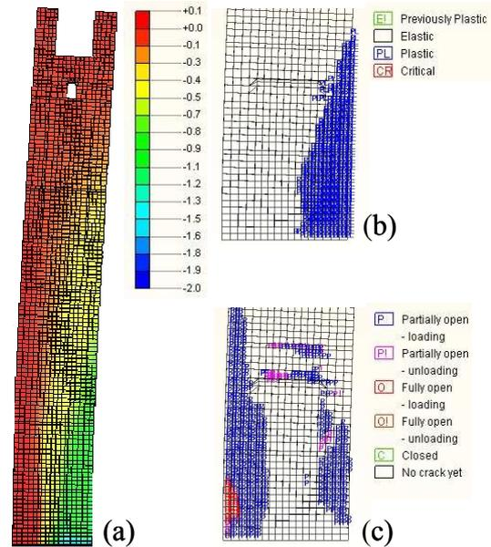
Figure 4: (a) Vertical stresses in the east façade at the collapse load step; (b) crushing and (c) cracking patterns in the critical zones at the base of the east façade at the collapse load step
