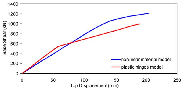
Figure 5: Comparison between the capacity curves of the nonlinear material model and of the plastic hinges model
