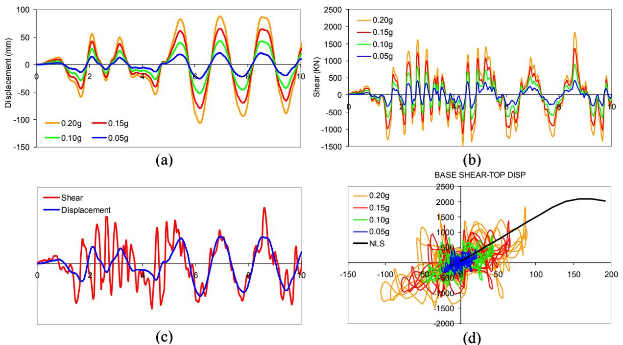
Figure 8: (a) Top displacement time history, (b) base shear time history and (c) relative qualitative comparison; (d) base shear-top displacement curves and pushover curve
