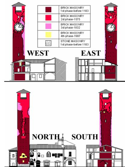
Figure 2: Construction phases of the tower
