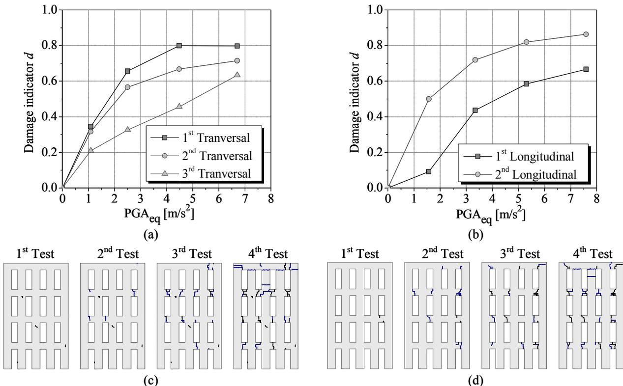
Figure 5: Vulnerability curves in the (a) transversal and (b) longitudinal direction and crack pattern of the (a) North and (b) South façade of the mock-up
