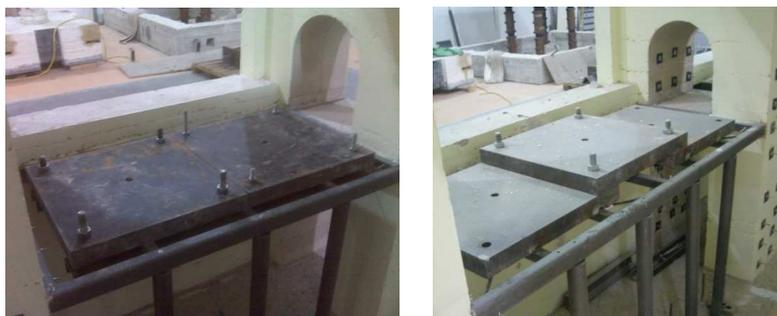
Figure 2: Additional masses in the physical model
