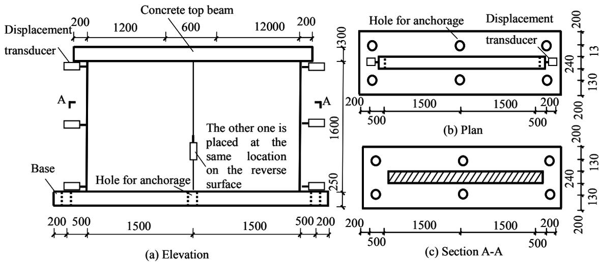
Figure 3: Dimension of the specimens and distribution of transducers
