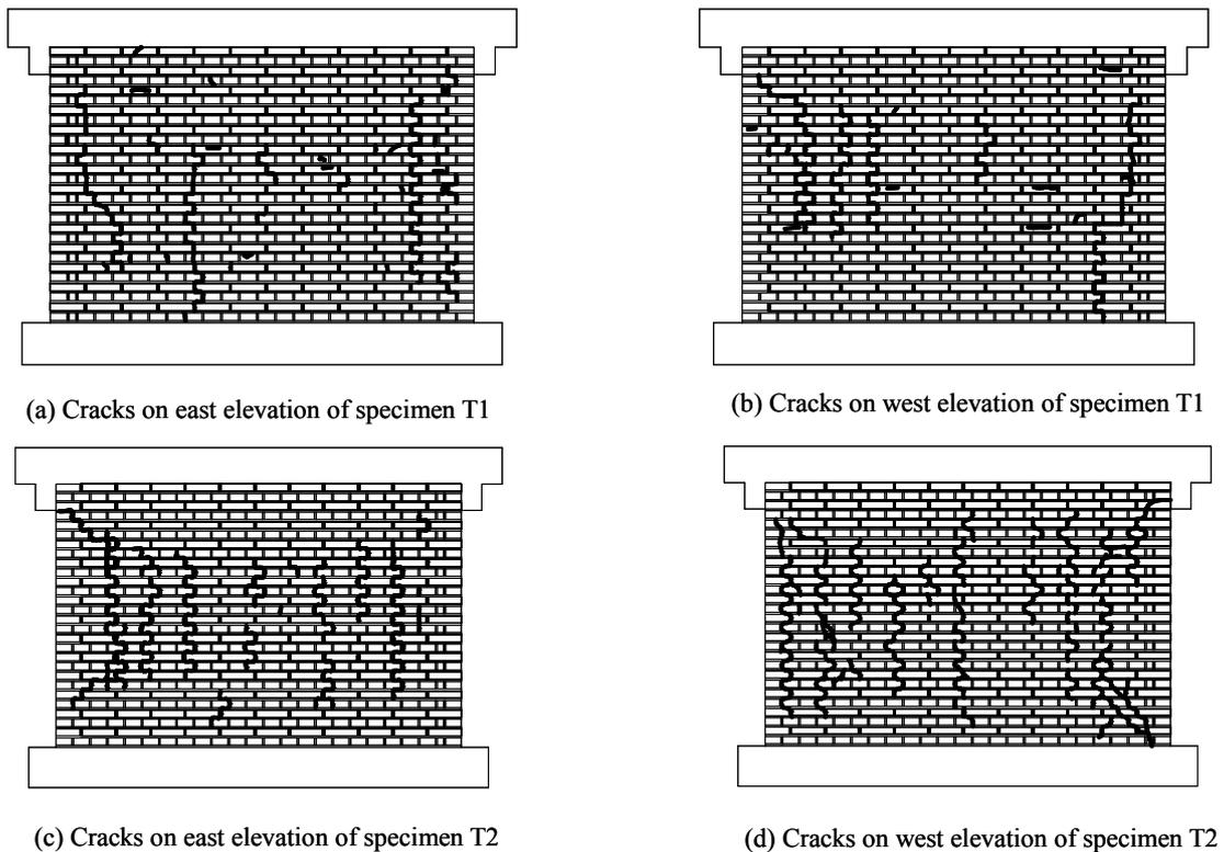
Figure 4: Cracks distribution of failure specimens
