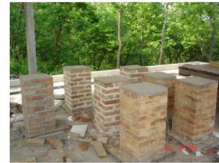
Figure 2: Masonry specimens
