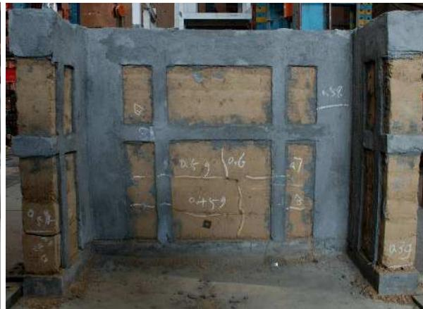
Figure 3: specimen B after test
