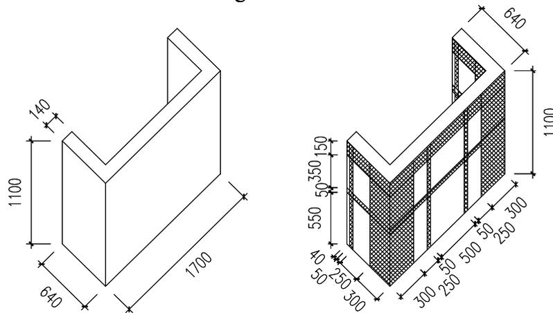
Figure 1: Dimensions (mm) and configuration of specimen A (left), B (right)
