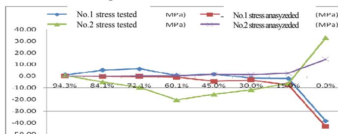
Figure 1: The comparison between test and theoretical stress value of bracket chord (Unit: MPa)
