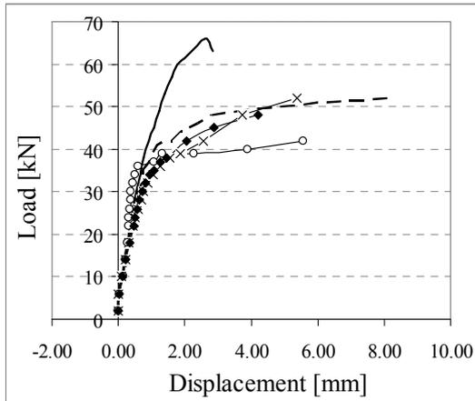
Figure 3: Comparison between traditional (continuous line) and hysteretic anchors
