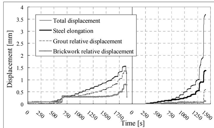
Figure 4: Relative displacements within the assembly for standard (left) and hysteretic (right) anchor
