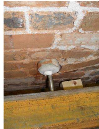
Figure 2: (a) Load-deflection curves of standard anchors and (b) example of pull-out failure
