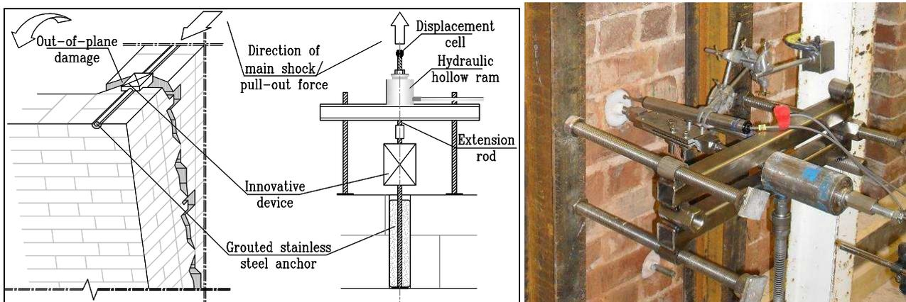
Figure 1: Real case application of cross tie and experimental set-up of pull-outs
