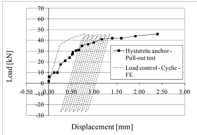
Figure 5: Load deflection curve - Comparison between pull-out tests and FEs
