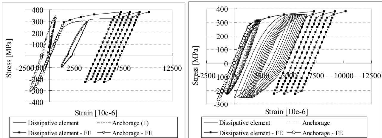
Figure 7: Stress-strain curves - FE models compared with static (left), and dynamic (right) tests
