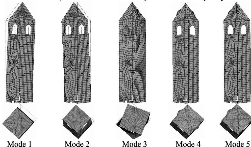
Figure 2: Vibration modes of the isolated tower
