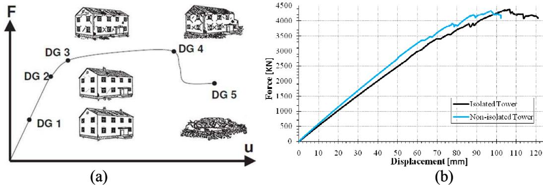
Figure 3: Results of the nonlinear analyses; (a) connection of the EMS-98 with a capacity curve (Lang 2002); and (b) capacity curves of the theoretical towers in their original state
