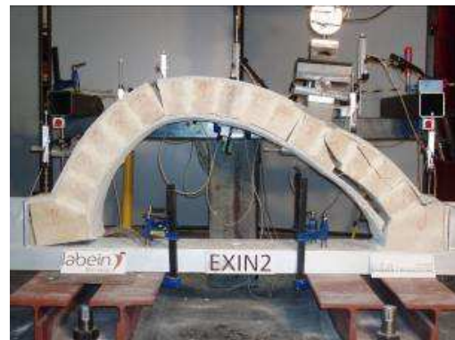
Figure 4: Tests on masonry arches. a) control arch, b) strengthened at both sides
