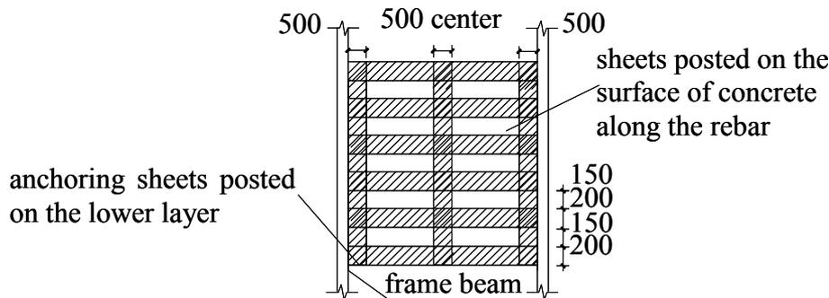
*Figure 5.1: Pasting diagram of CFRP on slabs (mm)*
