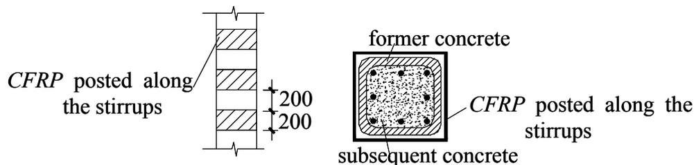
*Figure 5.2: Elevational and sectional drawings of CFRP on columns (mm)*
