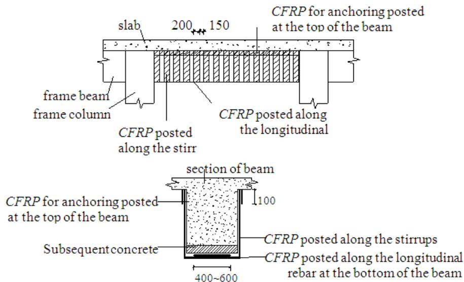
Figure 5.3: Elevation and sectional drawings of CFRP on beams (mm)
