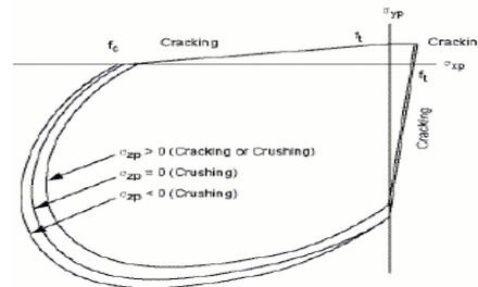
Figure 9: Willam-Warnke yield criterion at Concrete material in ANSYS
