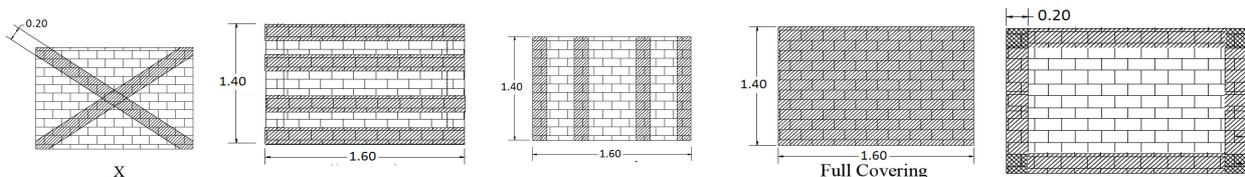
Figure 13: Different reinforcing patterns of the panel by FRP sheets
