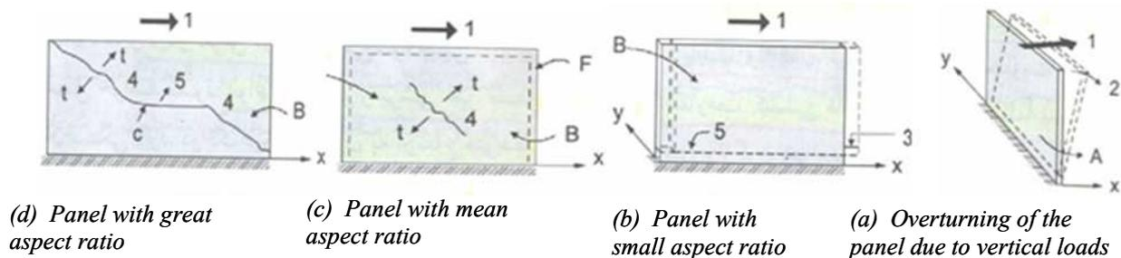
Figure 1: Cracking patterns at the panels
