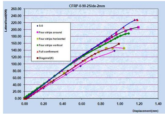
Figure 14: Lateral load-displacement of G3 with five FRP reinforcing method having fiber angle of 0-90 and thickness of 2 mm
