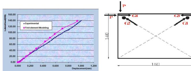
Figure 12: Lateral load- displacement at G3 direction
