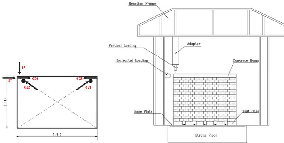
Figure 2: In plane shear test and displacement meter layout (Maheri 2008)
