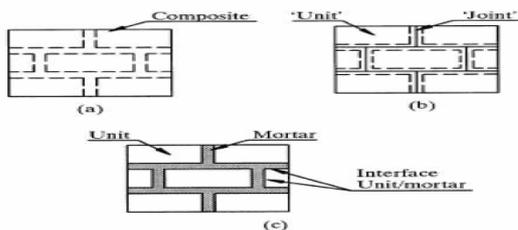
Figure 7: Macro modeling of the masonry panel
