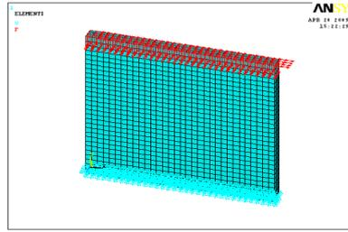
Figure 11: Finite element model of masonry panel and loading conditions
