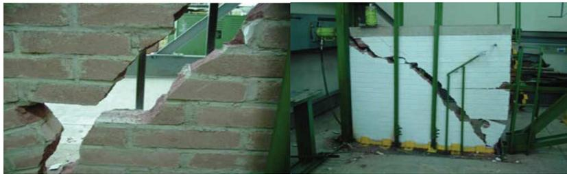
Figure 3: Loading conditions and failure of the masonry shear panel      Figure 4: Shear failure pattern as diagonal cracks
