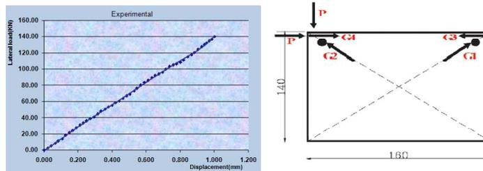
Figure 5: Load-Displacement curve for G3 lateral displacement transducer
