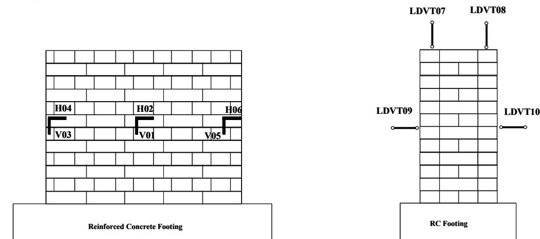
Figure 4: Test instruments
