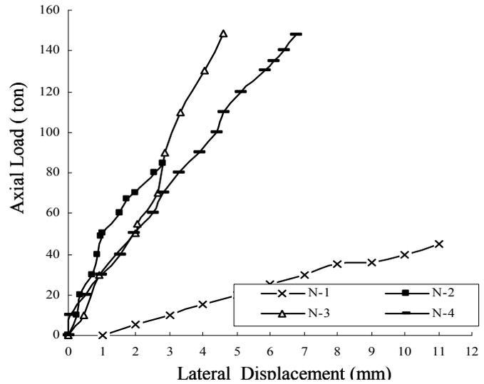
Figure 6: Load-lateral deformation responses of specimens
