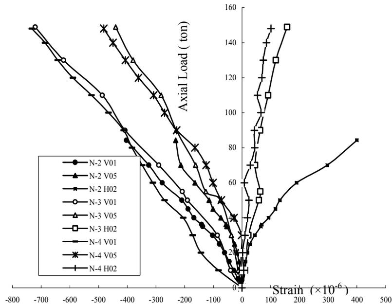
Figure 7: Strain developments on the masonry surface of specimens
