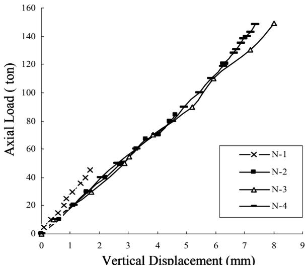
Figure 5: Load –vertical deformation responses of specimens
