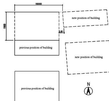
Figure 5: The old drugstore moving spot Figure 6: The old drugstore moving sketch map
