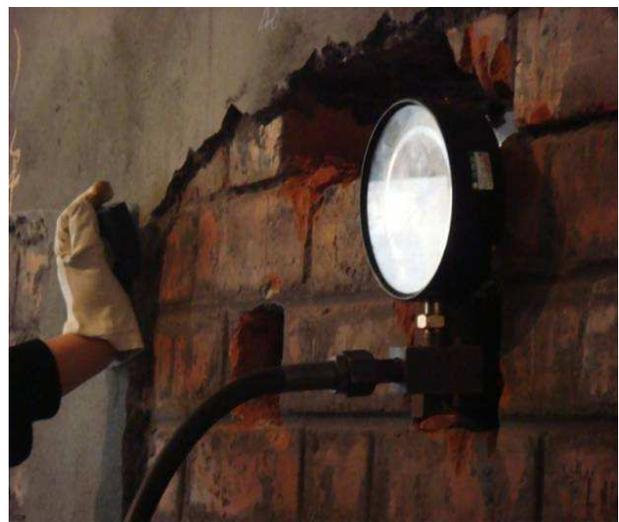
*Figure 6: shear strength test in situ after mortar replacement*
