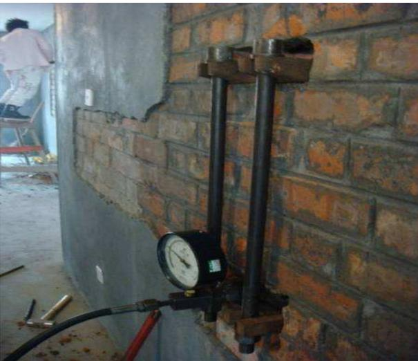
*Figure.5: bearing strength test in situ after mortar replacement*
