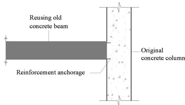
Figure 3: Reuse of original demolished concrete beam
