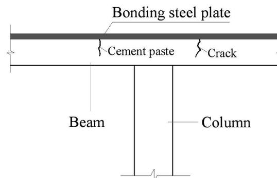
Figure 2: Crack repairing and beam strengthened by bonding steel plate
