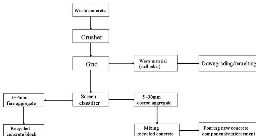
Figure 4: Recycling concrete waste
