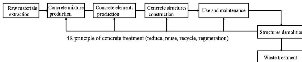
Figure 1: 4R principle in rehabilitation of concrete historic buildings
