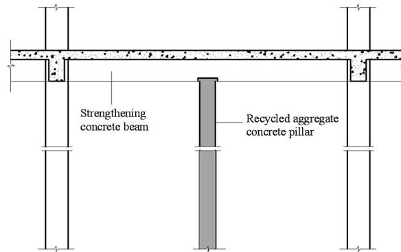
Figure 5: Additional fulcrum reinforcement
