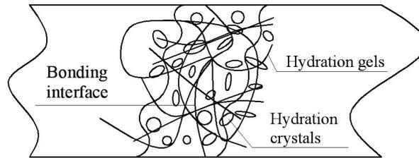
Figure 7: Bonding regeneration along interfaces between new and old concrete
