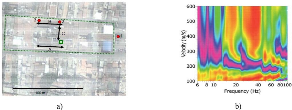
**Fig. 3** Parthasarathy temple (India): a) georeferenced feature map of the temple (green dotted lines), building analyzed with structural tests (green bold lines), seismic lines (black arrows, letters A to C) and Nakamura test locations (red dots, letters 1-3); b) MASW spectra showing phase velocity versus frequency for line A
