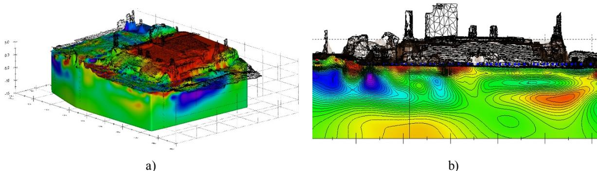
**Fig. 4** Marte Ultore temple (Italy): preliminary results of Electrical Resistivity Tomography, 3D and 2D view respectively (courtesy of G. Morelli, Geostudi Astier)
