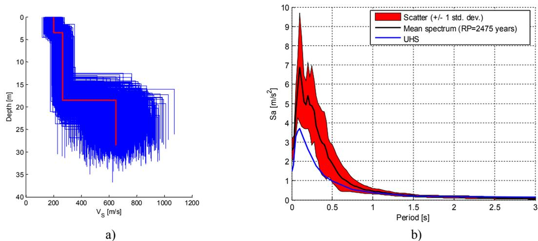
**Fig. 5** Stochastic ground response analyses at the Indian site: a) random profiles obtained using the Latin hypercube sampling technique (the red line represents the mean profile) and b) mean spectrum (black line) plus/minus one standard deviation (red area) at the surface and the UHS obtained from the PSHA (blue line)
