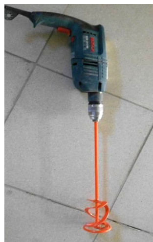
Fig. 2 The mixer blade used in experimental work
