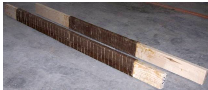
Fig. 7 G3 and G4 beams repaired with the bio-composite system
