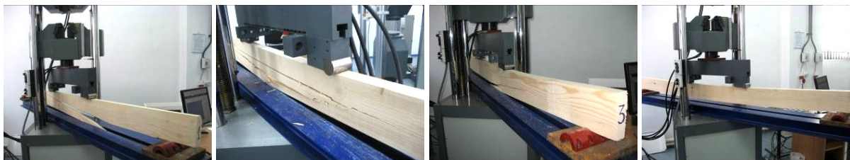
Fig. 6 Four points bending test of timber beams; test setup and failure modes
