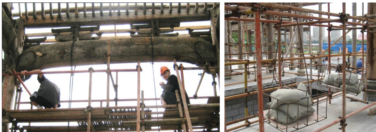
Fig. 2 Steel lifting cage and cable connection position of beams under static loading
