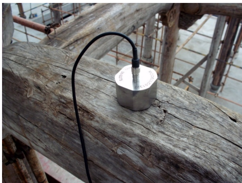
Fig. 3 Lance piezoelectric type accelerometers for measurement of acceleration
