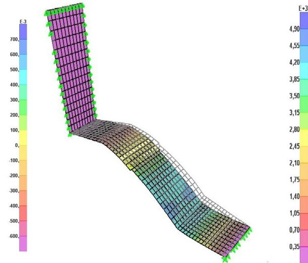
Fig. 6 Deformed shape of the bridge SAP2000 model
