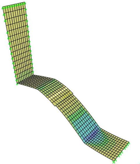
Fig. 5 SAP2000 finite element model
