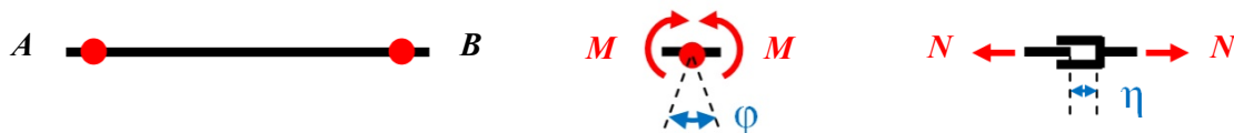
Fig. 2 Schematic representation of a beam finite element with plastic joints (at edges A and B )
