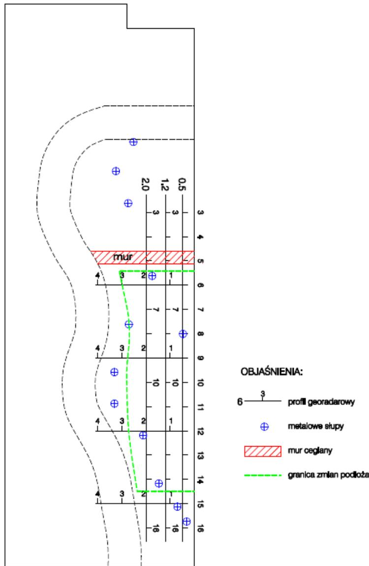
**Fig. 2** The results of GPR researches of the Rotunda of the Holly Virgin Mary at the Wawel Hill. Cracow Geodetic Company. Scale 1:100
