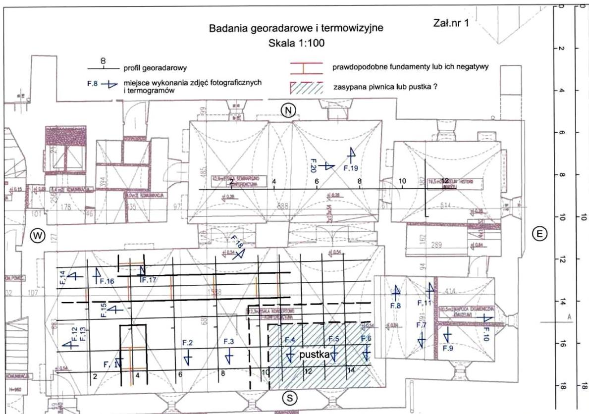
**Fig. 1** The results of GPR researches of the Castel of Sobotka Gorka. Cracow Geodetic Company
