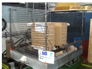
Fig. 2 Wall specimens (SAWR and SAWV) on shake table
