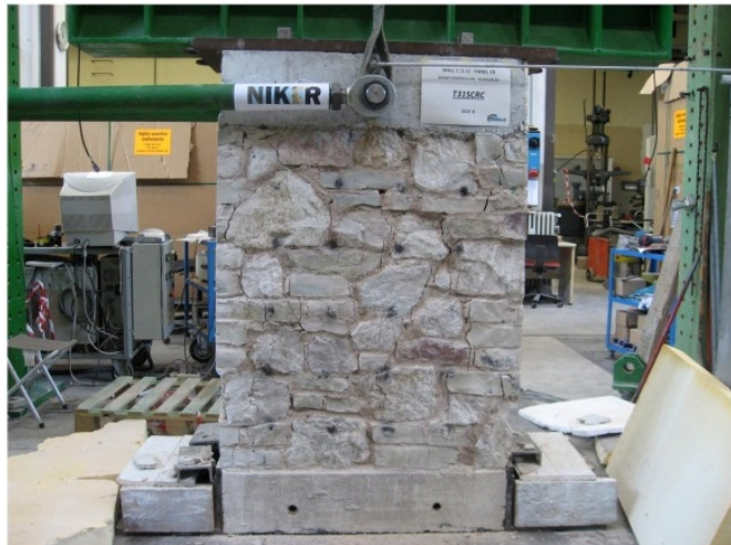
Fig. 3 Finite element model of the panels: mesh, boundary conditions and applied loads on the numerical simulation of the shear-compression tests. Numerical model (left). Experimental test of panel C8 (right)
