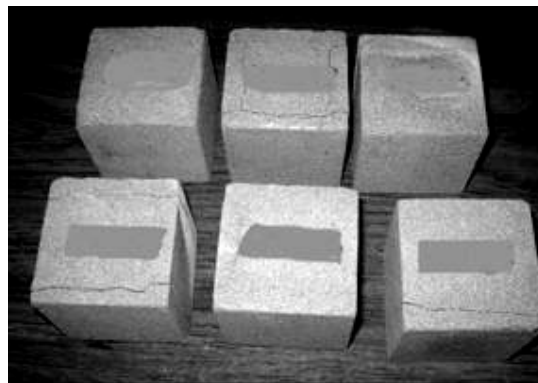
Fig. 4 Apc12 specimens after the salt crystallisation cycles (cubes of 40 mm edge)
