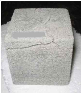
Fig. 3 Apc8 specimen after 15 SC cycles (40 mm edge)
