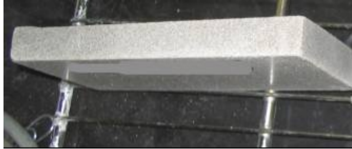
Fig. 7 Apc2 specimens after SO 2 cycles with solution B (120 × 60 × 10 mm dimensions)
