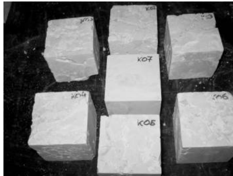
Fig. 2 Calcarenitic specimens (6) after salt crystallization test and the not altered (KO7). The weight loss of the specimens was of 1% but the alteration is evident
