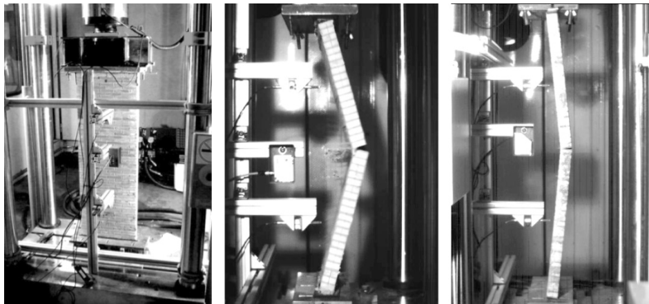
Fig. 1 Wall loading arrangement (left), and typical failure modes (middle and right)
