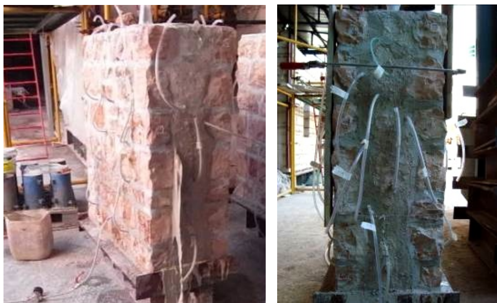
Fig. 9 Walette 4. Application of grouts
