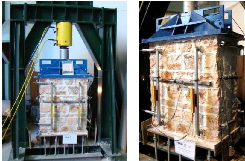
Fig. 1 Test setup and instrumentation of wallettes subjected to compression.
