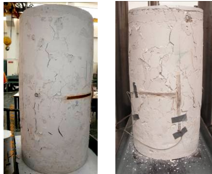
Fig. 3 Failure mode of grouted infill material in compression.
