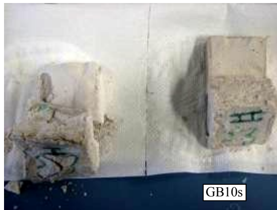
Fig. 5 Photographs of grout specimens after six (6) cycles of exposure
