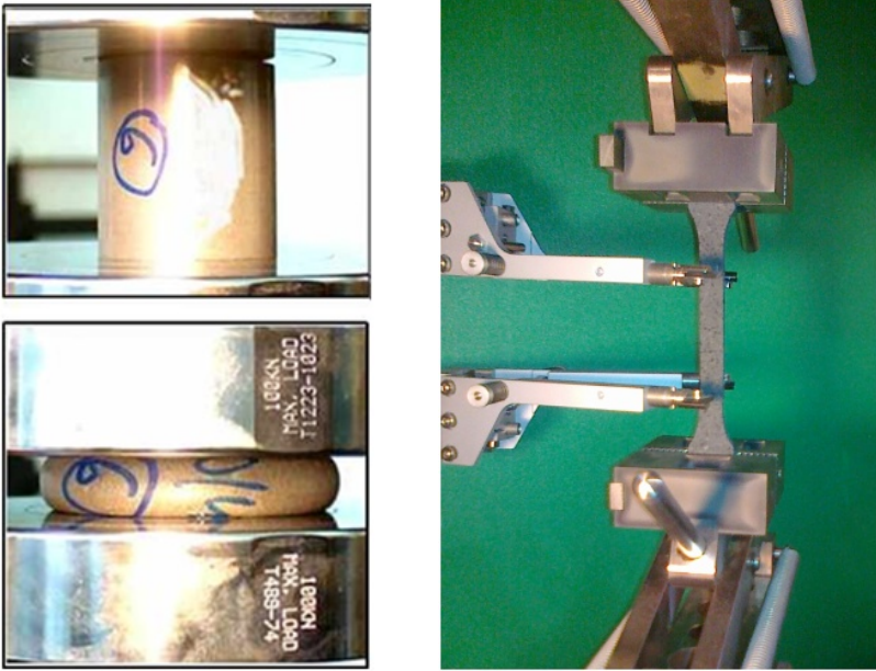
Fig. 2 Compressive (left) and tensile (right) setup with the tested specimens of the polymer PM
