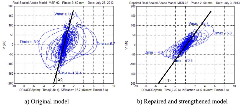
Figure 10. Base shear vs. top displacement curves for second testing phase (D = 60 mm)
