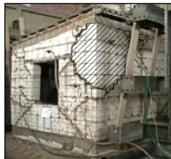
a) Damaged full scale model
