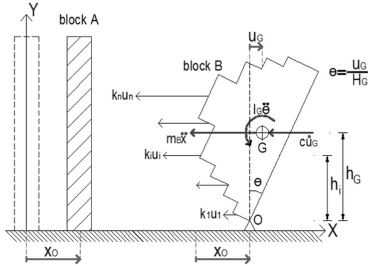
Figure 12. Free body diagram of block B
