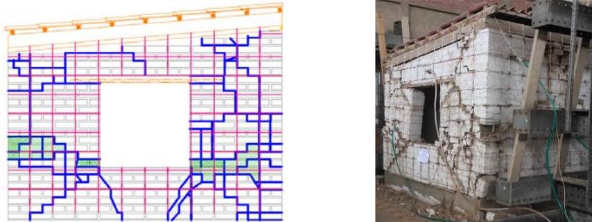
**Figure 8.** Sketch of damage pattern and general view of the model after all shaking phases.
