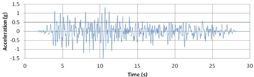
Figure 2. Shaking table acceleration recorded in a test with  $D = 130$  mm peak command displacement.
