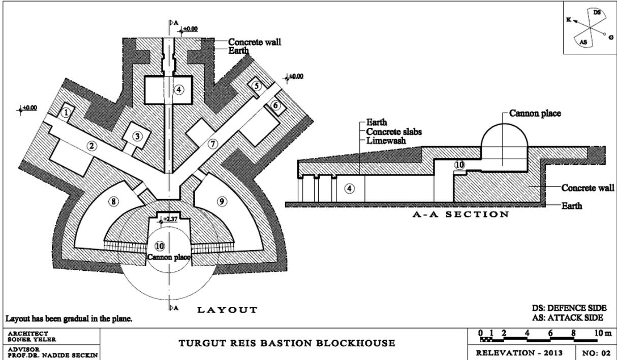
Figure 5: The example of concrete construction system, Blockhouse of Turgut Reis Bastion, 2013 [8]
