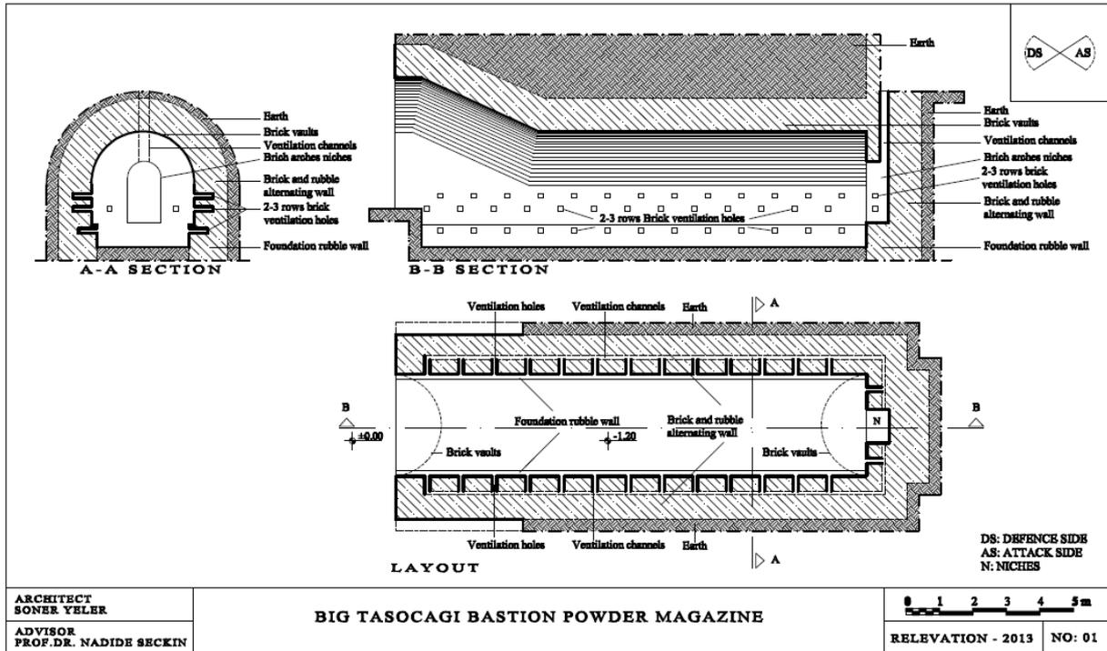
Figure 4: The example of masonry construction system, Big Tasocagi Bastion, 2012 [8]
