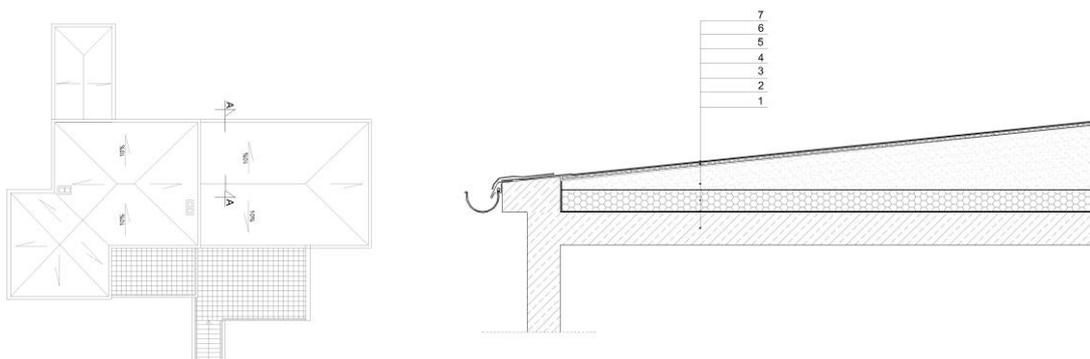
Figure 9: Single family house designed by Emil Lange, WuWA model Werkbund estate built in Wroclaw (former Breslau) in 1929. Flat roof plan and section of flat roof (renovation proposal): 1 – original roof construction 26 cm high, 2 – steam insulation, 3 – Styrodur thermal insulation 15 cm thick, 4 – insulation fibre, 5 – concrete decrease layer with light expanded clay aggregate , 6 – mortar bed, 7 - heat applied roofing felt (2 layers). Drawn by A.Tomaszewicz.
