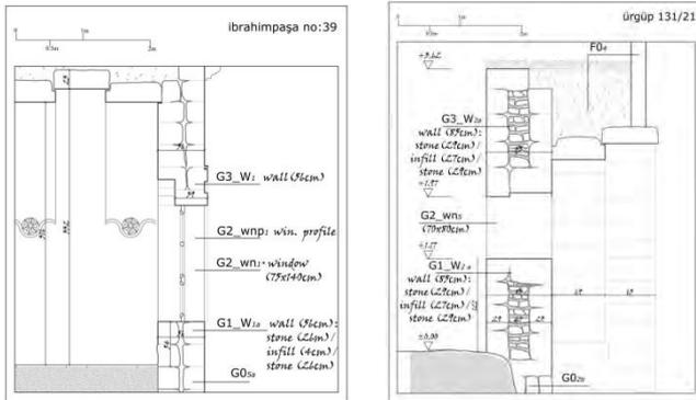
Fig. 7-8, Wall type 1a (cut-stone/infill/cut-stone)- Wall type 2a
