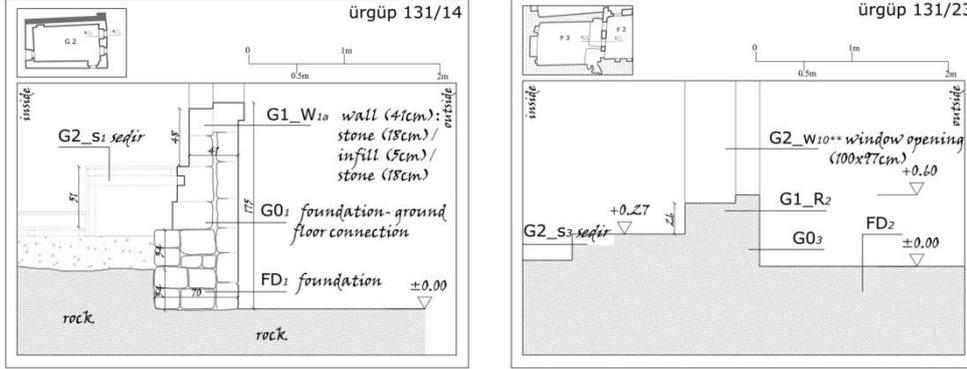
Fig. 2-3, Detail of foundation type 1- Detail of foundation type 2
