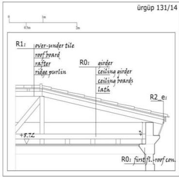
Figure 22, Timber roof on cornices
