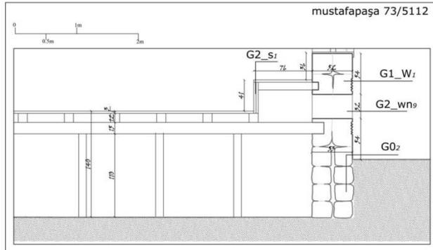
Figure 21, Elevated timber floor and *sedir* (Mustafapaşa, block/lot: 73/5112-1)
