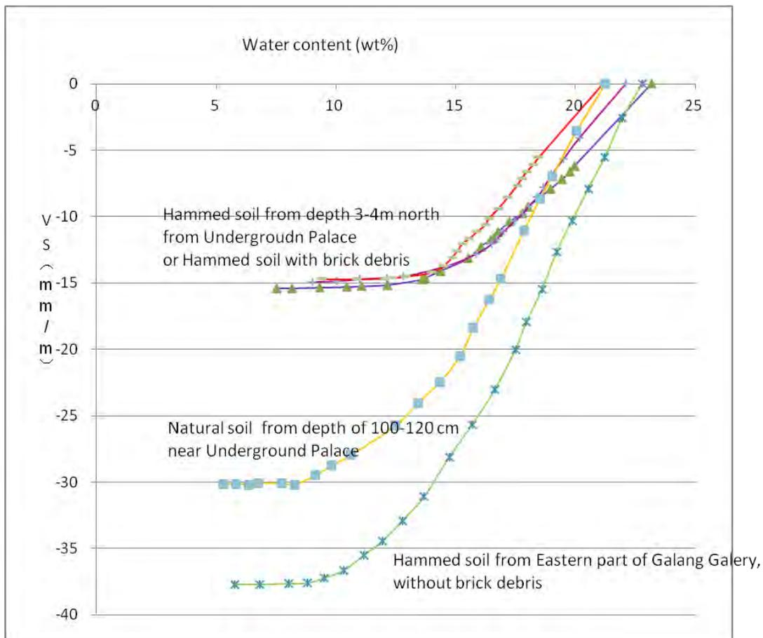
Figure 3: Shrinkage curves of various earths from Grand Bao En Temple, Nanjing
