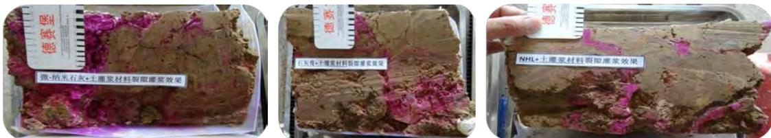
Figure 10: Cross section and carbonation of injection grouts based on limes
