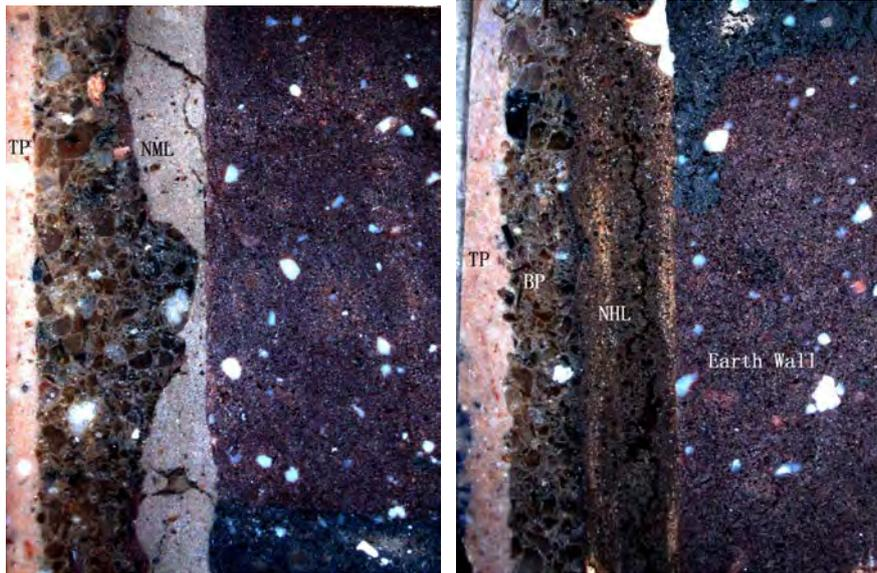
Figure12: Microscopic photos of the injection grouts (TP= old top lime plaster, BP=old base lime plaster, NML=new microlime injection grout, NHL= new natural hydraulic lime grout)
