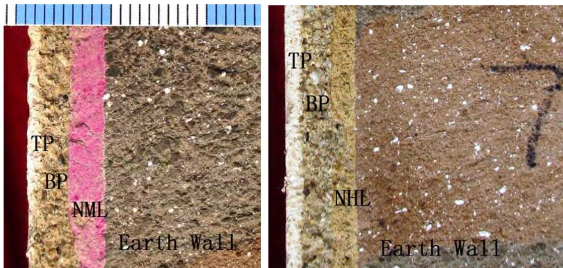
Figure 11: Carbonation of 2 injection grouts to attached lime plaster
