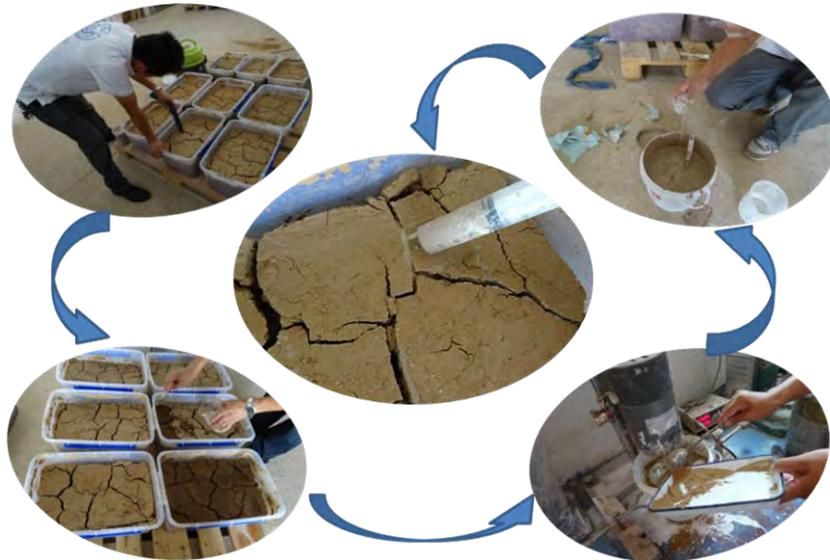
Figure 9: Performance testing of three types grouts into earth cracks simulated to ruins
