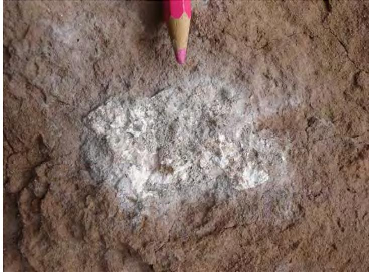
Figure 6: Earth sample taken from City wall top, which restored around 1979 showing migration of lime into earth
