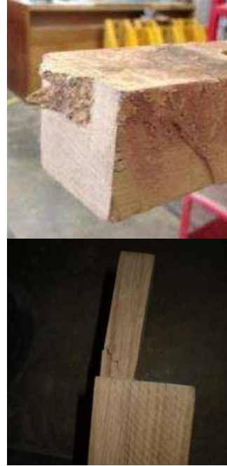
Figure 14: Failure of tenon in A2 (top) and A1 (bottom)
