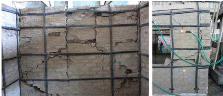
Figure 4: The cracking pattern after the test on the module (from Charleson [3]).
