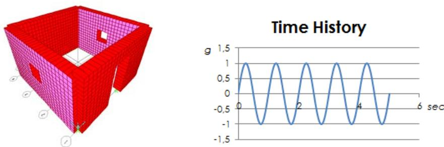
Figure 12: Model for dynamic analyses and input acceleration time history.
