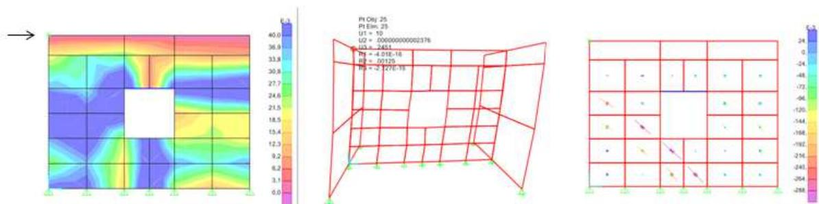
Figure 8: Principal tensile stresses [Mpa].
