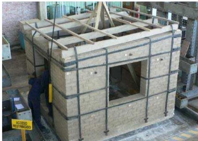
Figure 3: Module tested on a shaking table (from Charleson [3]).
