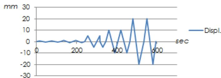
Figure 10: Displacement history of the cyclic test.
