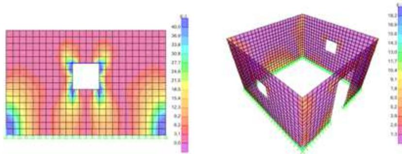
Figure 13: Principal tensile stresses on the left and  $s_{23}$  on the right [MPa] for 0,4g of PGA.
