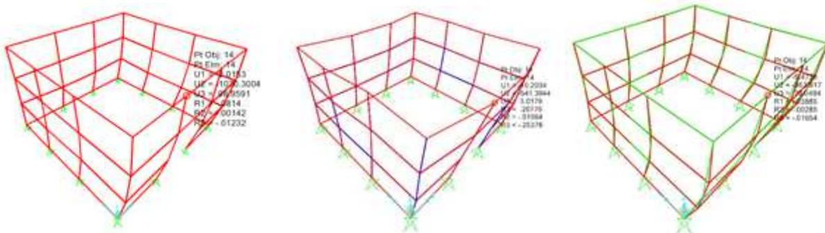
Figure 14: Maximum displacements for: the unreinforced model, the bamboo reinforced model and the used car tyre straps mesh reinforced model.
