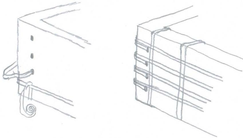
Figure 2: Steps in the process of reinforcing (from Charleson [3], redrawn).
