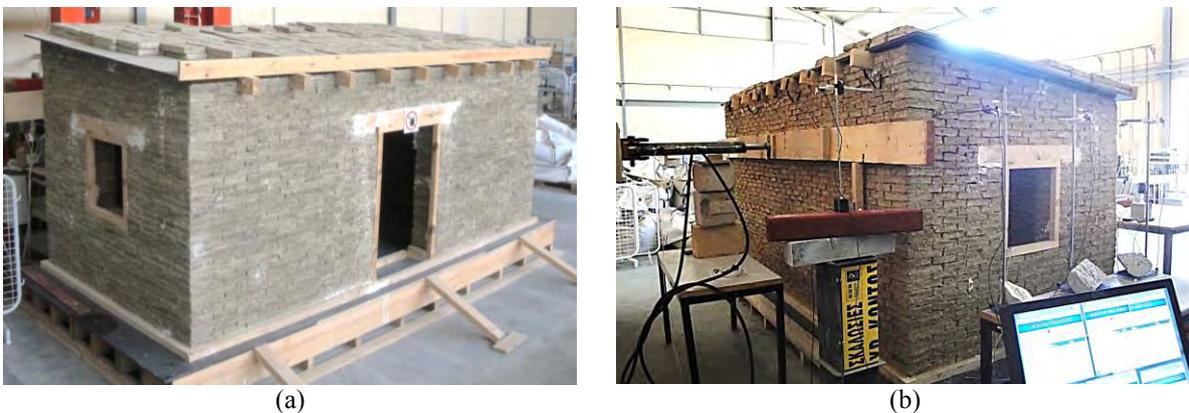
Figure 1: (a) The 1:2 scaled adobe building tested at the Structures Laboratory of the University of Cyprus. (b) The hydraulic jack and the timber beam used for imposing lateral loads on the structure's rear wall.
