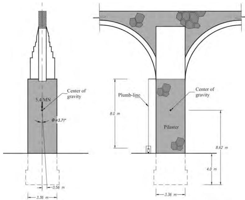
Figure 10 Geometric model to define the maximum tolerable rotation
