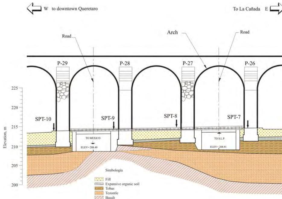
Figure 3 Stratigraphy between pilasters 26 - 29
