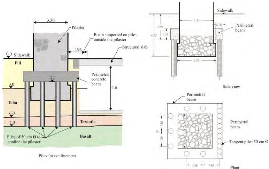
Figure 4. Confinement of the pilasters
