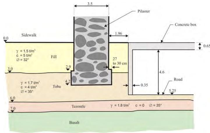
Figure 5. Foundation of the pilasters
