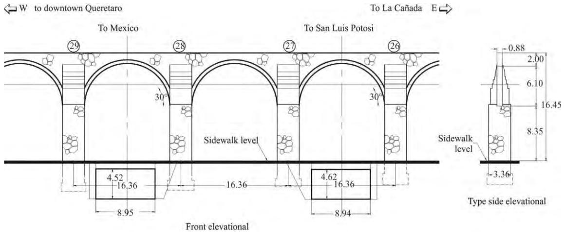
Figure 1 View of arches 25 to 29, dimensions in m
