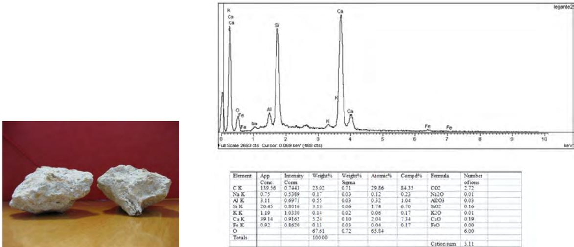
Figure 6. Results from the EDS analysis of a portion of the binder. Silica peaks reveal the binder hydraulic properties.
