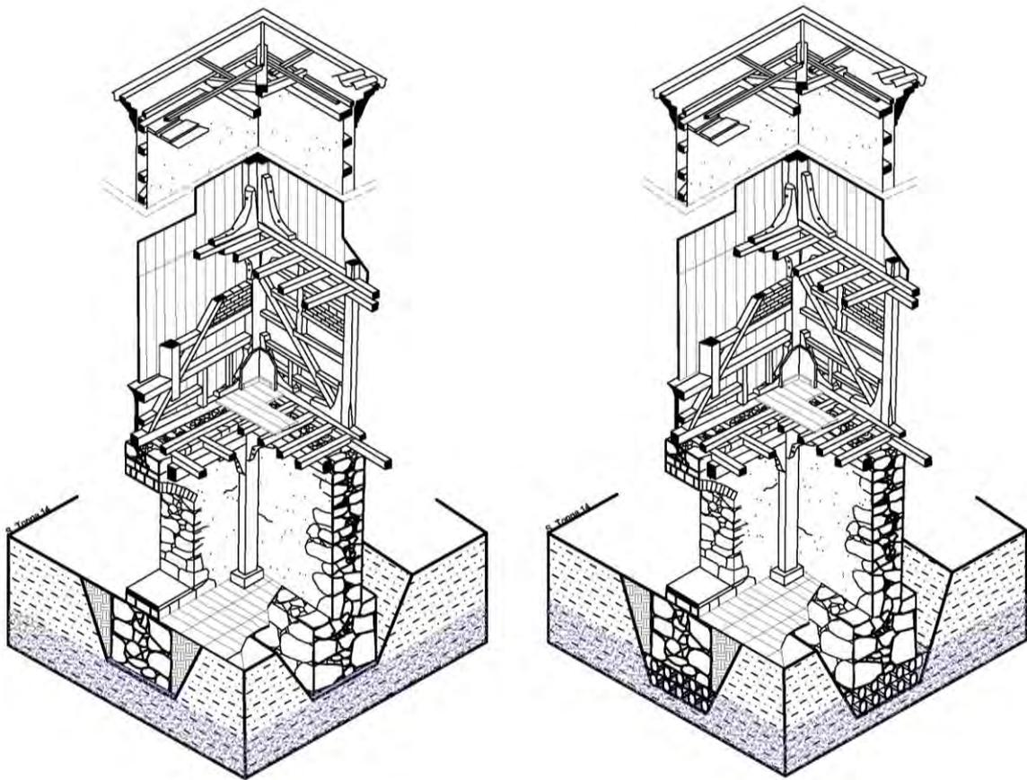
Figure 7. The foundation structures present in the Lefkada traditional buildings. On the left Foundation wall with pozzolana in the mortar, on the right with the timber grid.
