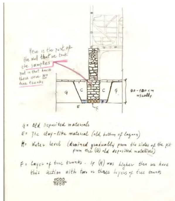
Figure 2. The foundation system according to K. Katopodis.
