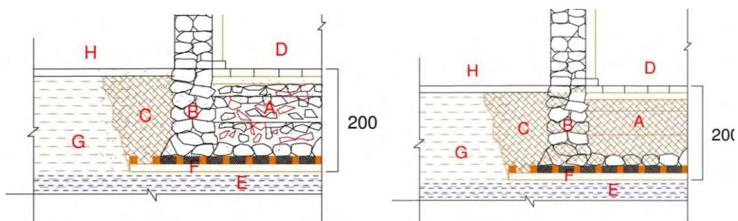
Figure 1. Initial assumptions on the foundation system.
