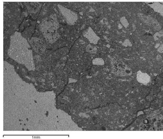
Figure 5. The mortar specimen as seen with the petrographic optical microscope.
