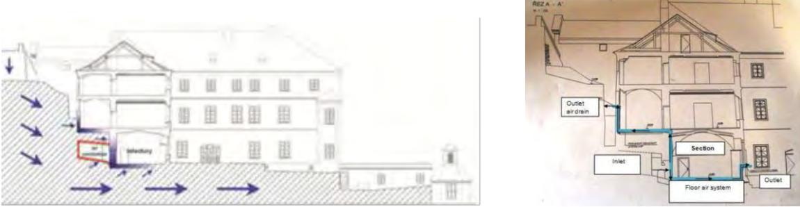
**Figure 3 – Cross-section showing groundwater flow (left); air ventilation system (right)**
