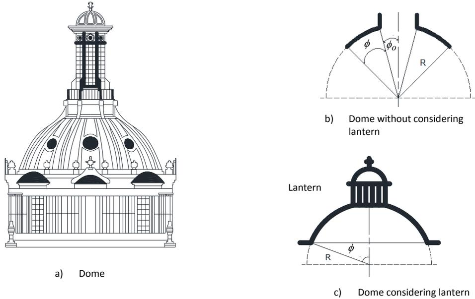
Figure 6: Geometric data to calculate the stresses in domes
