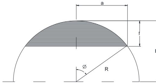
Figure 5: Geometric data to calculate the stresses in a recessed hemispherical vault
