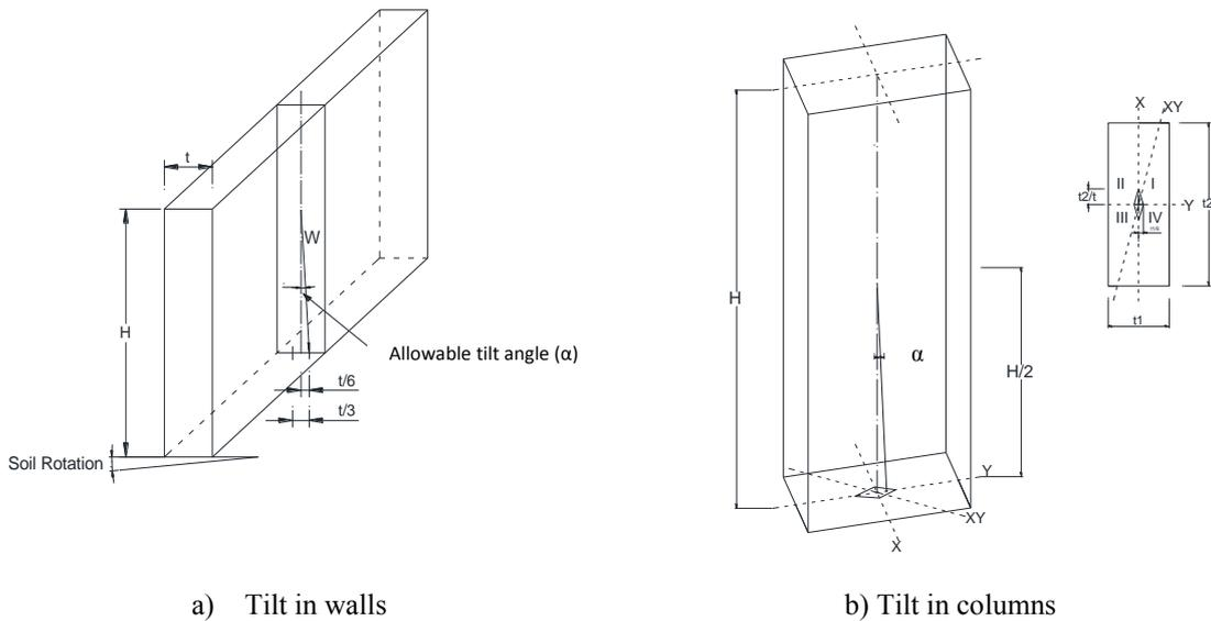
Figure 4: Allowable tilt angle according to Heyman
