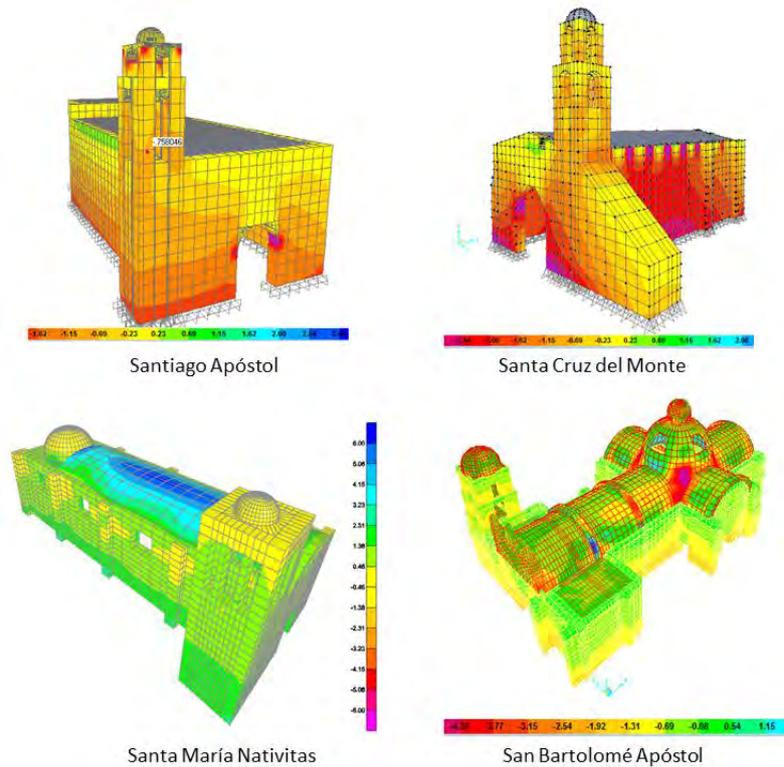
Figure 8: Finite element models of the parishes
