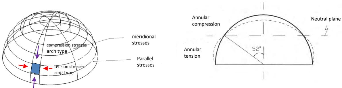
Figure 3: Internal stresses, meridional and parallel, in a hemispherical dome
