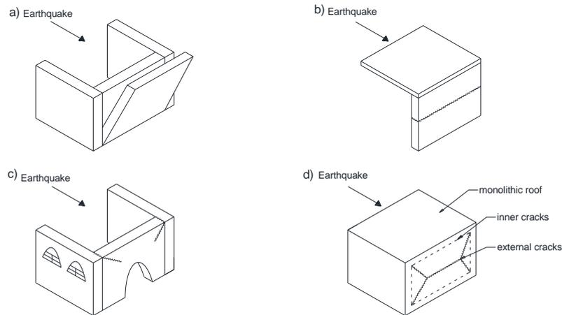
Figure 2: Failure modes in walls due to the earthquake [2]
