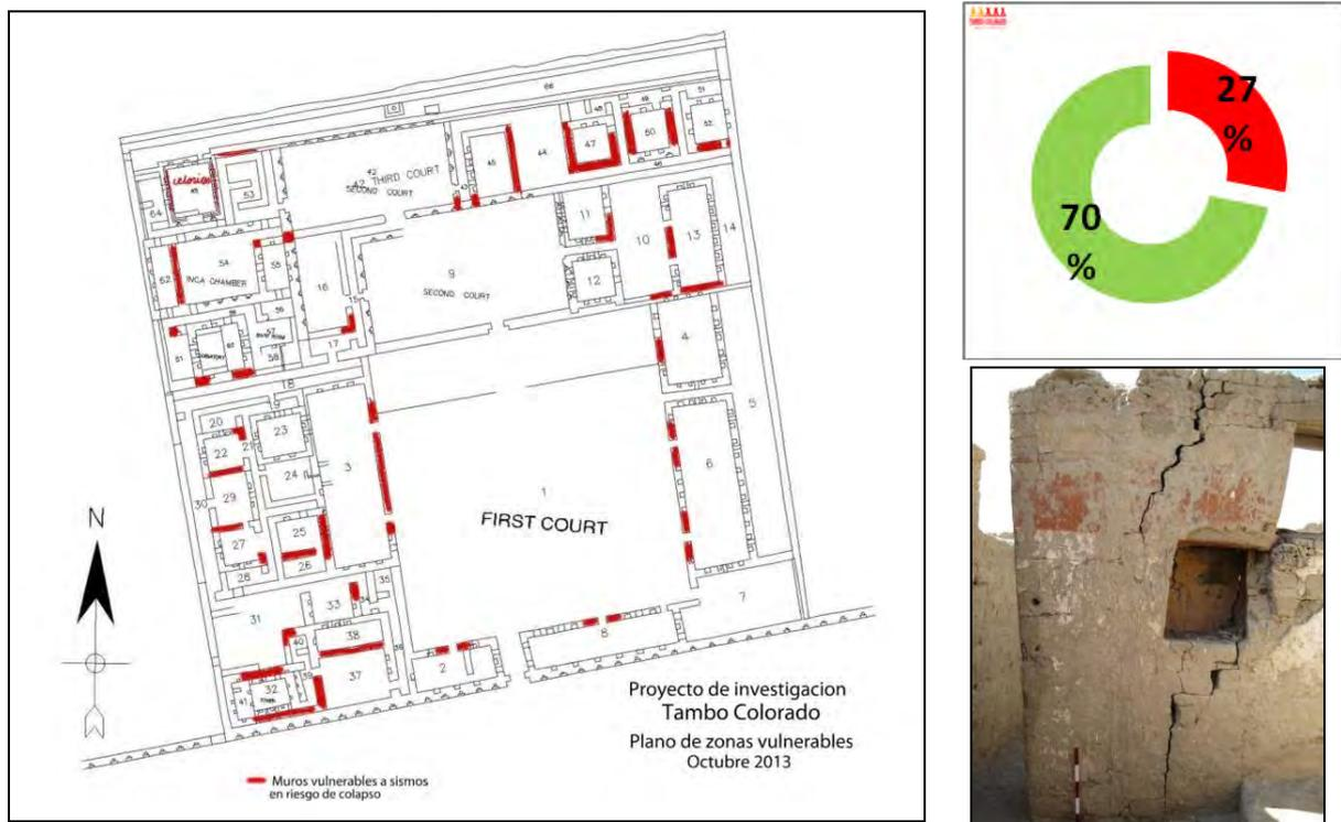
Figure 9. North Palace I vulnerability it shows enclosures with walls in risk of collapse (© PRTC, 2013).
