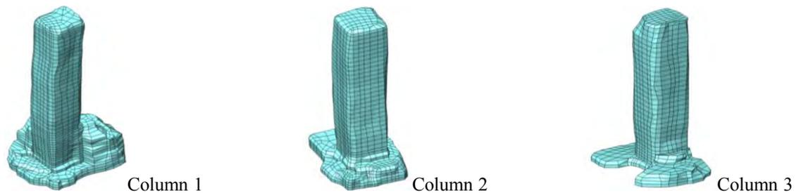
Figure 13: Finite element models of columns at Huaca de la Luna.
