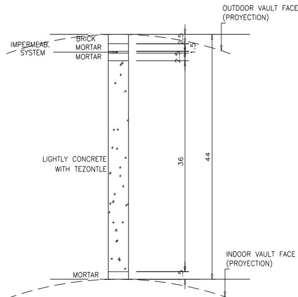
Figure 10: Typical vault construction system.
