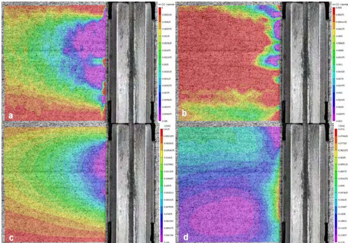
Figure 5: Full-field results obtained by DIC and computed on the left side of the jaws; a) strain in the direction of applied force ( $\epsilon_{xx}$ ); b) Strain in the direction perpendicular to applied force ( $\epsilon_{yy}$ ); c) displacement in the direction of applied force ( $u$ ); displacement in the direction of applied force ( $v$ )
