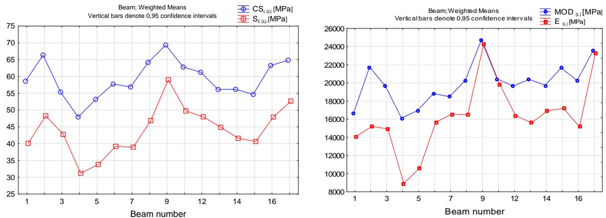
Figure 3 left: Compressive strength  $S_{C(L)}$  and conventional compressive strength  $CS_{C(L)}$  parallel to grain for individual beams (pushing jaws in the hole apart); right: elastic modulus  $E_{(L)}$  and modulus of deformability  $MOD_{(L)}$  parallel to grain for individual beams (pushing jaws in the hole apart)
