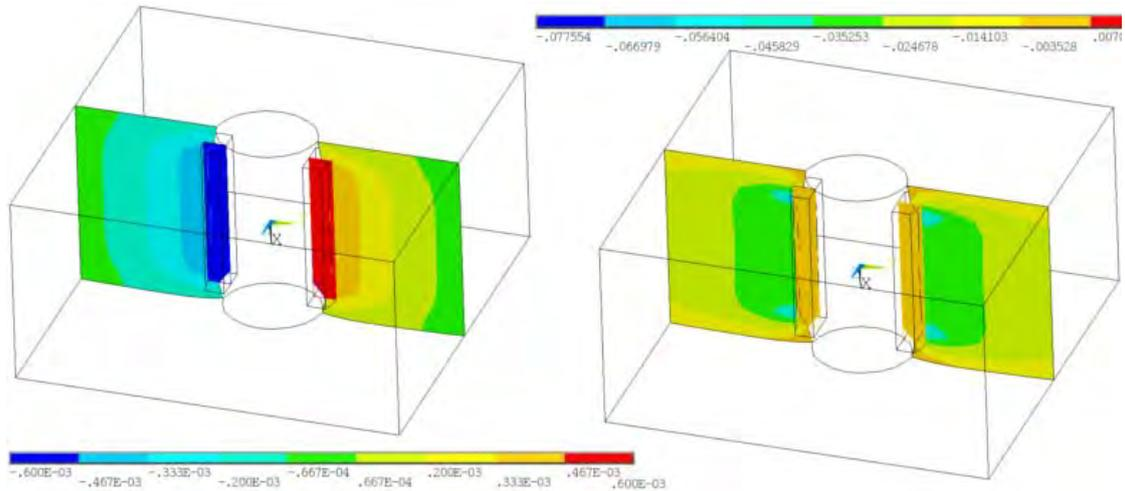
Figure 4: results from the FEA; left – displacement in the direction of applied force ( $u$ ); right – strain in the direction of applied force ( $\epsilon_{xx}$ )
