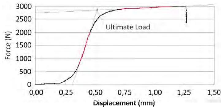
Figure 2: an example of the device output and sketch of determination of the conventional strength
