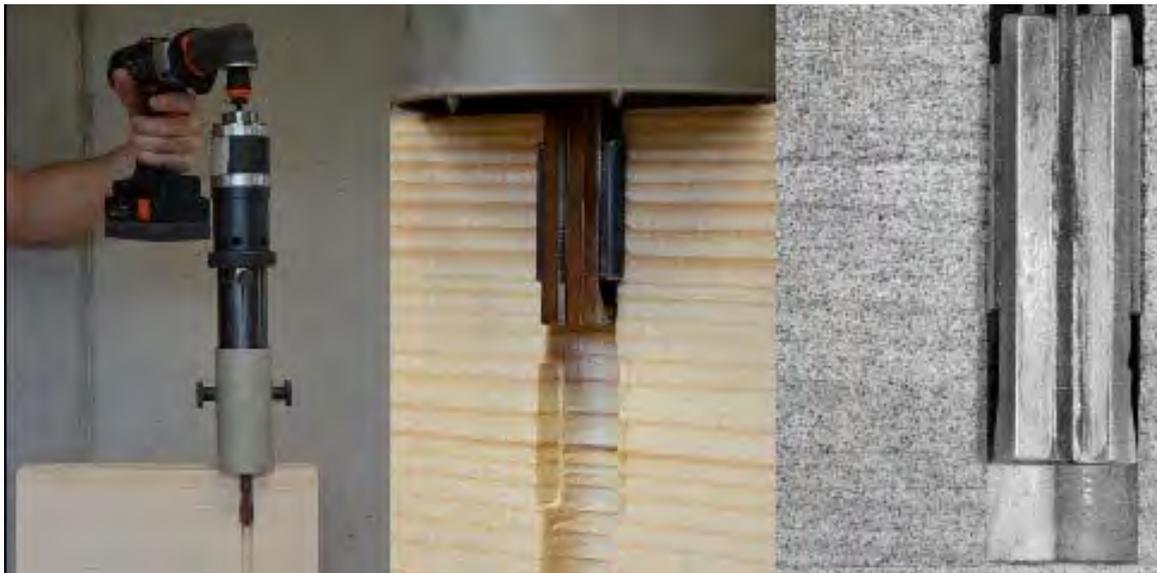
Figure 1: left – overall view of the newly designed device; center – detail of the drawbar with the wedge and rounded jaws; right – example of random two-component pattern for DIC analysis
