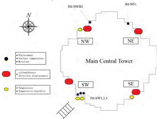
Fig.3 Sensor position in Bayon
