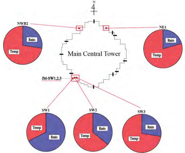
Fig.8 Temperature in each measurement spot, comparison of the rain influence degree
