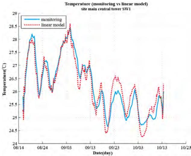
Fig.7 Comparison between calculation result and observation of the surface temperature in the chronological order
