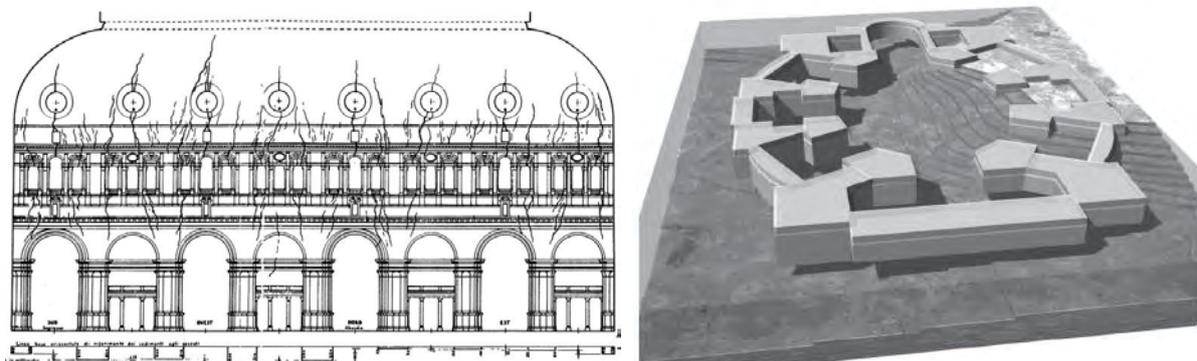
Figure 2: Cracking pattern on the dome (left side) and axonometric view of the foundations (right side).
