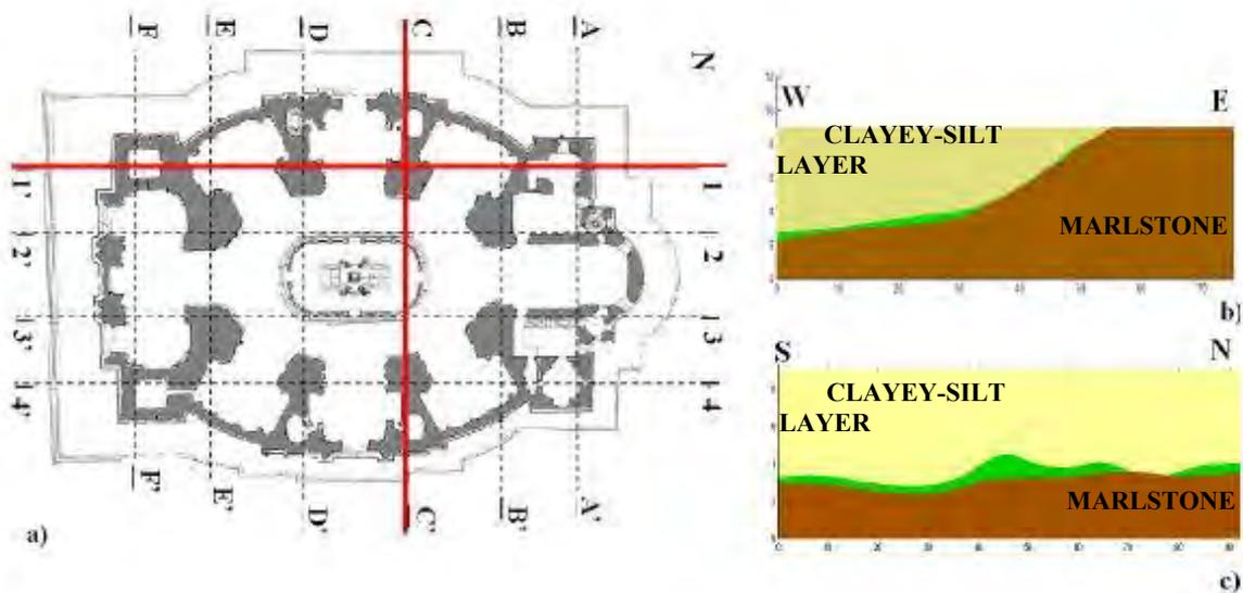
Figure 3: (a) position of the generated vertical cross-sections; (b) section C-C' West-East; (c) section 1-1' South-North [3].
