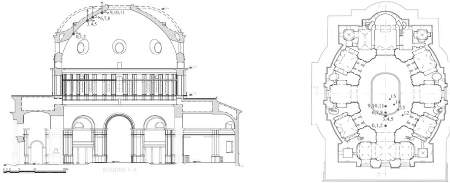
Figure 6: Arrangement of accelerometers and geophones in one of the various setups.
