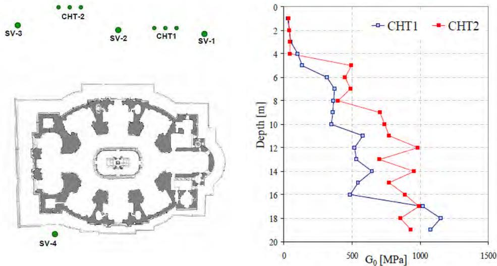
Figure 4: Position of cross-hole tests (CH) performed in 2004 during the geotechnical investigations campaign.
