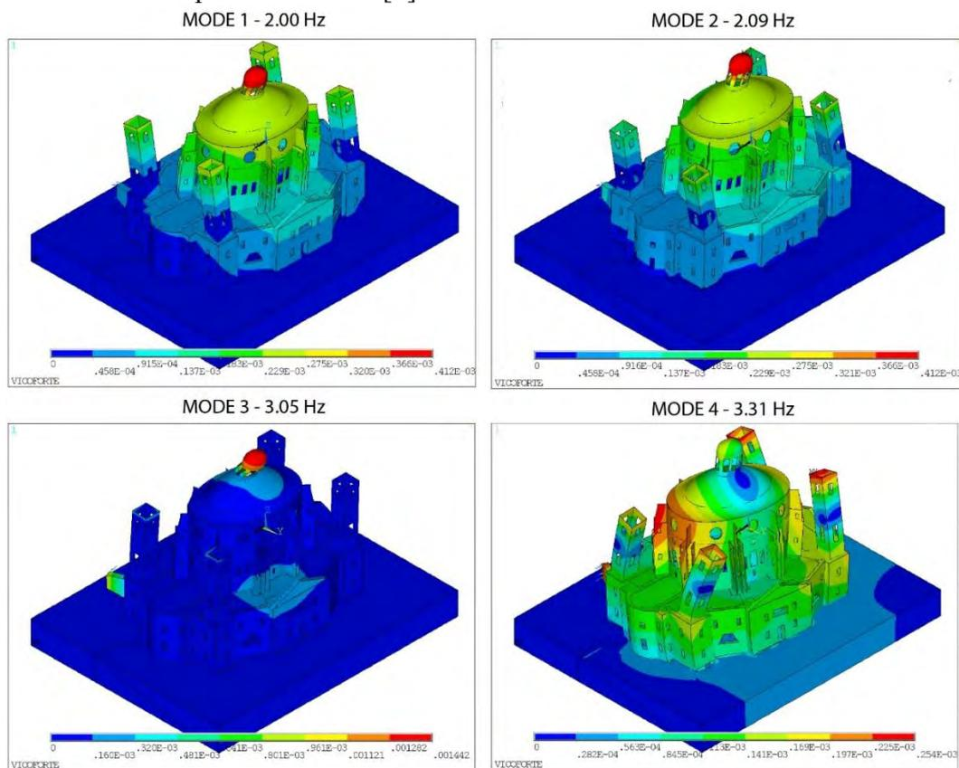
Figure 8: The first four FE modes: the two first flexural modes, the second flexural (or the first mode of the lantern) and the first torsional mode (the frequencies are already referred to the calibrated model).
