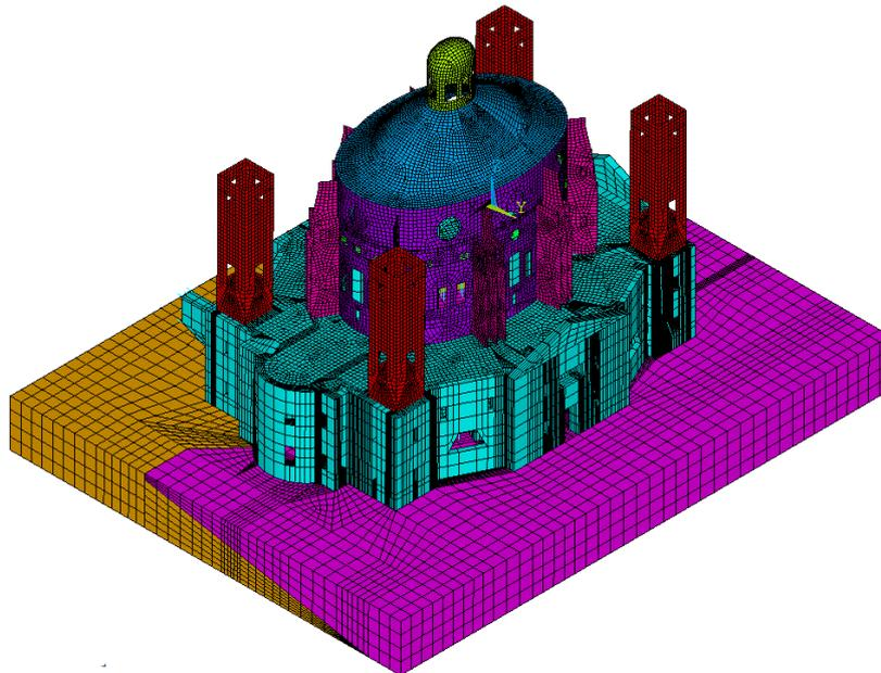
Figure 7: The finite element model inclusive of foundation soil (clay-silt in purple and marlstone in light brown). The other colours identify the different material used for the different macro-elements within the model.
