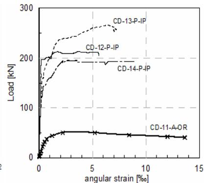
Figure 10: Curves of the shear stress-angular strain response for stone masonry panels (Diagonal compression test method, L'Aquila).
