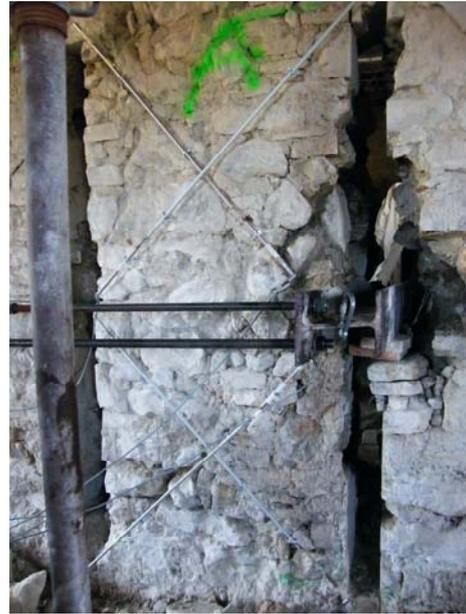
Figure 2: Shear-compression test.
