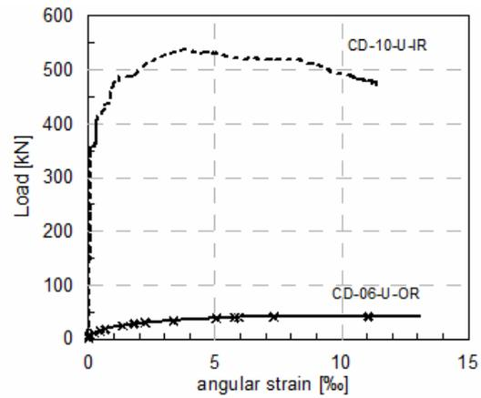
Figure 7: Curves of the shear load-angular strain response for stone masonry panels for the 19th-century masonry typology.
