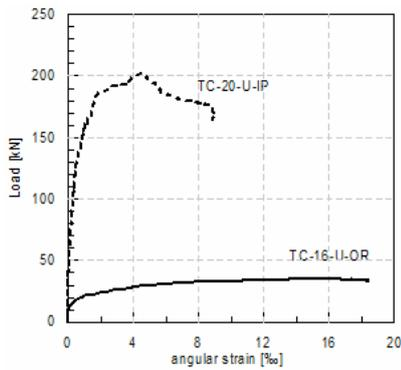
Figure 8: Curves of the shear load-angular strain response for stone masonry panels (shear compression test method, Colle Umberto) for the 20th-century masonry typology.
