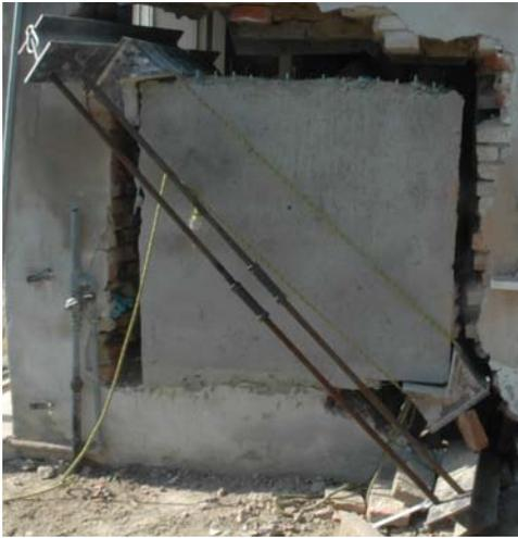
Figure 1: Diagonal compression test.
