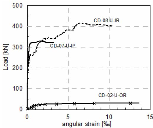
Figure 6: Curves of the shear load-angular strain response for stone masonry panels for the 20th-century masonry typology.
