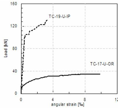
Figure 9: Curves of the shear load-angular strain response for stone masonry panels (shear compression test method, Colle Umberto) for the 19th-century masonry typology.
