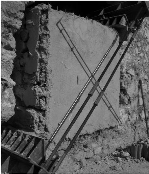
Figure 11: A panel subjected to diagonal compression test retrofitted with ferrocement.
