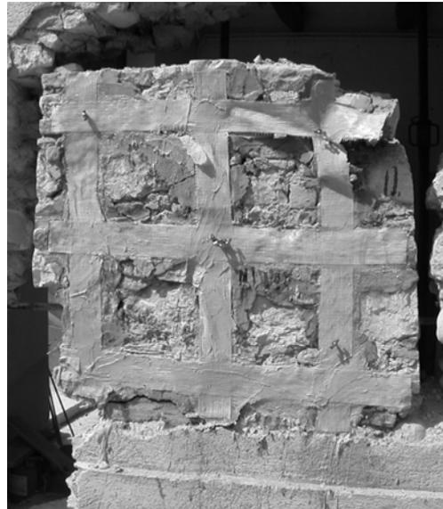
Figure 12: A panel subjected to diagonal compression test retrofitted with GFRP sheets applied with an epoxy resin.
